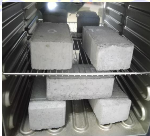
Gambar 3.4 Pengujian Daya Serap Air Paving Block
