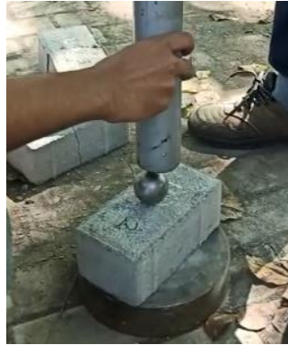
Gambar 3.4 Pengujian Beban Impact Paving Block
