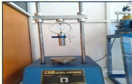
**Gambar 3.11** Alat Uji Penetrasi CBR Laboratorium
