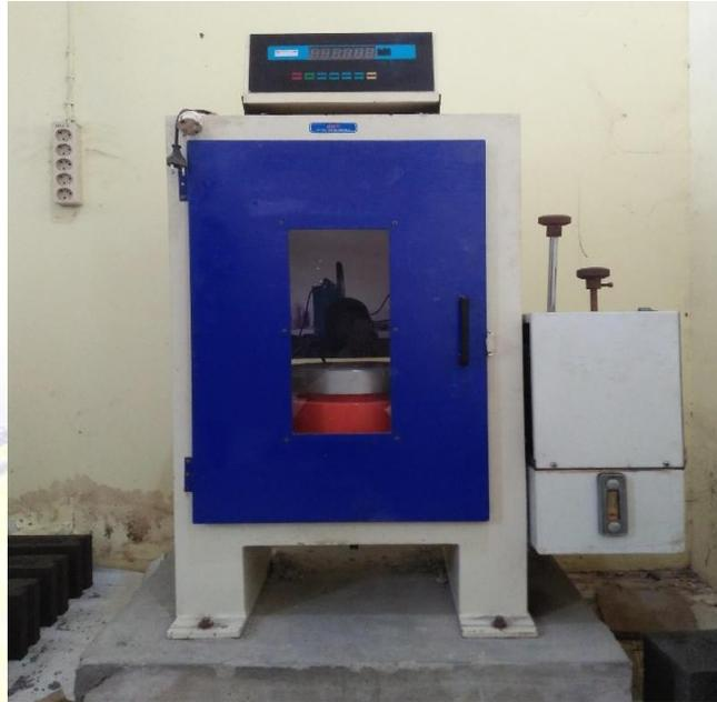
**Gambar 3.14** Alat Uji Kompresi (*Compression Tester/CTM*)
