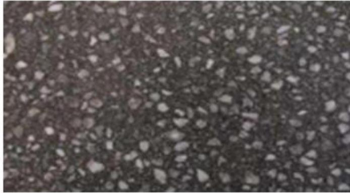
Gambar 2.18 Agregat Aus
