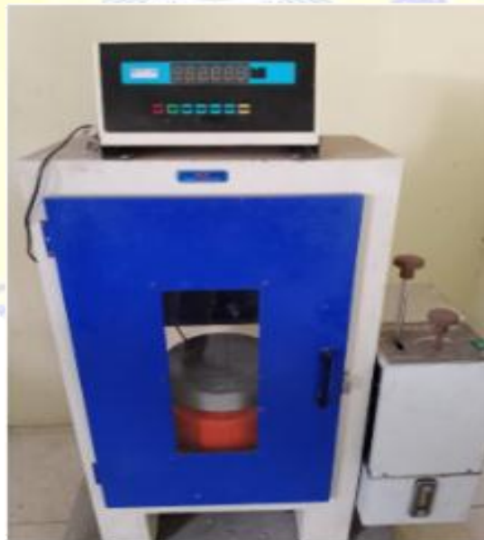
Gambar 3.6 CTM ( Compression Testing Machine )
