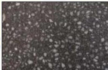
Gambar 2.18 Agregat Aus.
