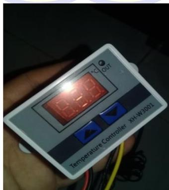
Gambar 12. Temperature Controller XH-W3001
