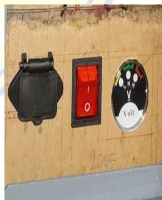
Socket charger, switch on-off, voltmeter
