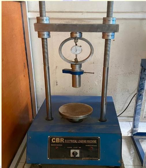
**Gambar 3.18** Alat uji penetrasi CBR laboratorium
