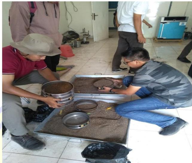
Gambar, 3.2. Analisa Saringan Agregat (Sumber: Data Hasil Penelitian)
