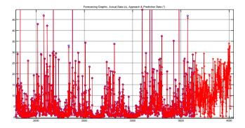
**Figure 3.** Results of daily rainfall prediction from actual data using two hidden layers
