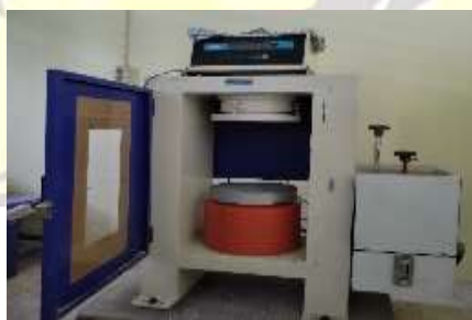
Gambar 3.11 CTM (Compression Testing Machine)
