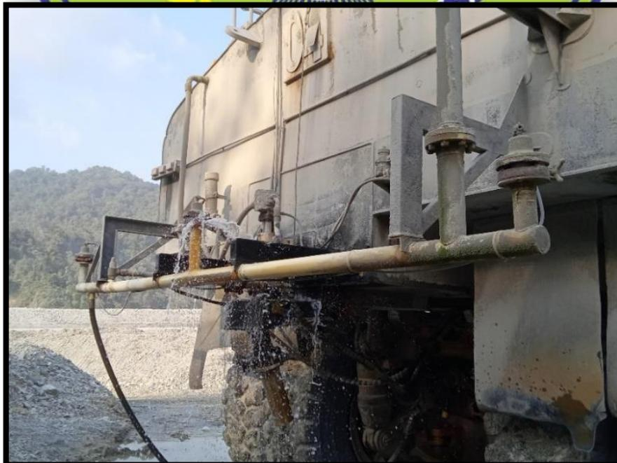
Gambar 3.3 *Spray Pada Unit Water Truk*
