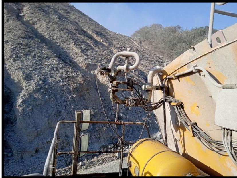
Gambar 3.5 *Water Cannon Pada Water Truk*
