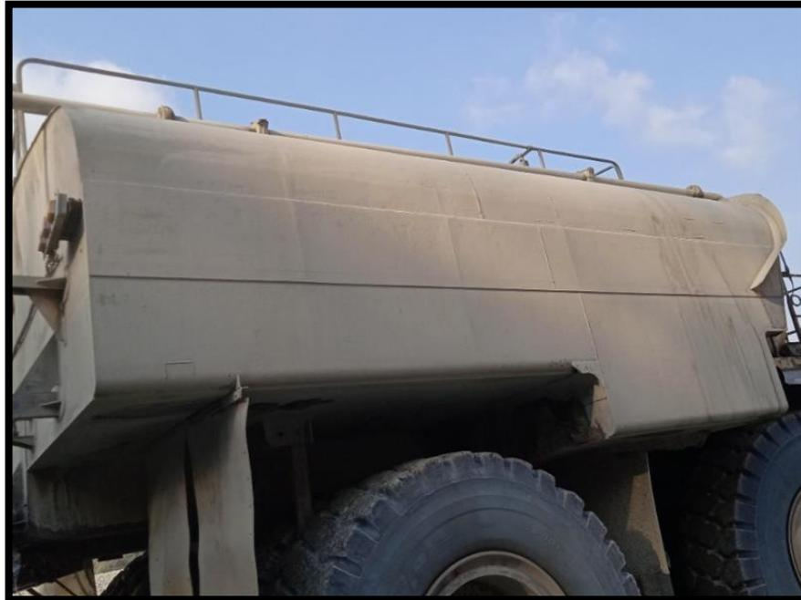
Gambar 3.2 *Tank Unit Water Truk*
