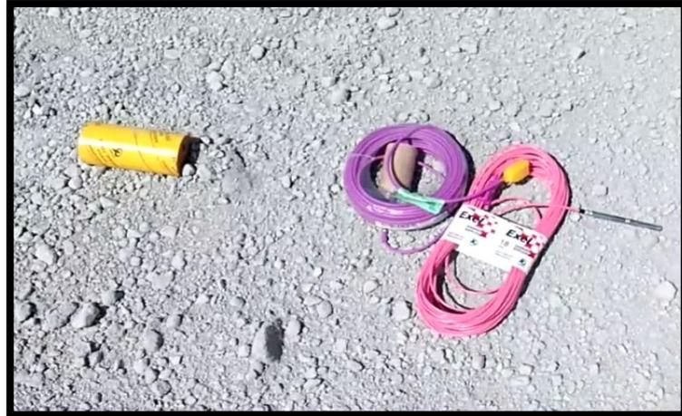
Gambar 2.14. Elektronik detonator, *booster*, dan *non-electric* detonator
