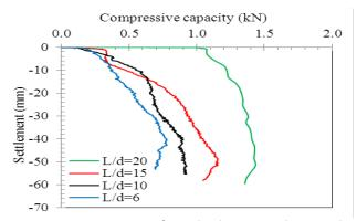
Figure 7 Compressive capacity for single pile versus settlement under different L/d ratio
