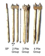
Figure 4 Group pile models: L= 200 mm; d= 10 mm
