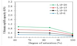
Figure 6 Ultimate uplift capacity for single pile versus degree of saturation of soil under different L/d ratio
