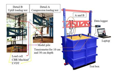
Figure 2 Setups of model piles for compression and uplift loading tests [18]
