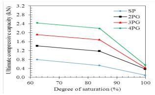
Figure 12 The pile group's ultimate compressive capacity versus degree of soil saturation
