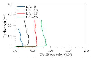
**Figure 5** Single pile uplift capacity versus displacement under the different ratio of L/d
