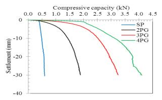
Figure 11 Pile group compressive capacity versus the settlement under various pile number in a group
