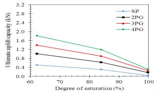
Figure 10 Ultimate uplift capacity for the pile group versus the degree of saturation
