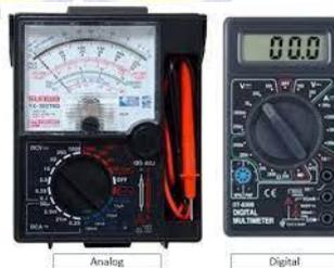
Gambar 7 . Multimeter
