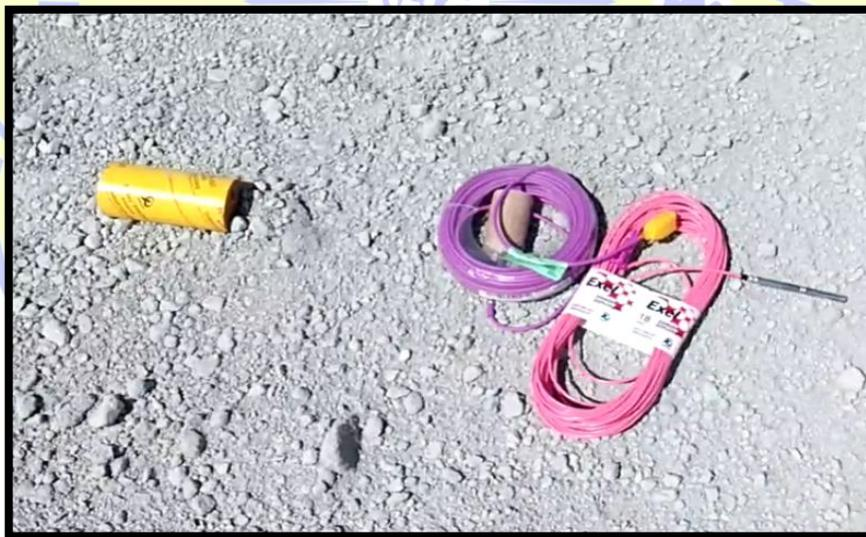
Gambar 2.13. Elektronik detonator, *booster*, dan *non-electric* detonator
