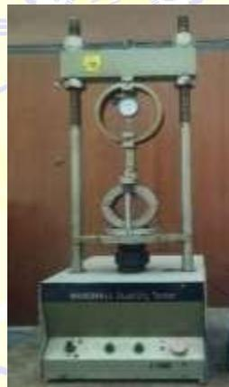
Gambar 3.20. *Marshall test*
