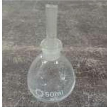
Gambar 3.2. *Piknometer* labu
