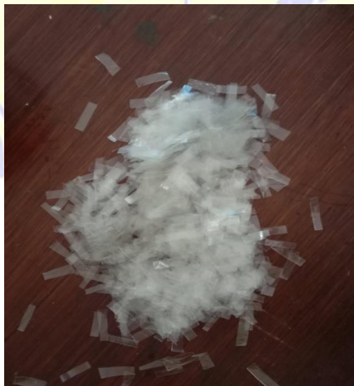
Gambar 3.6 Sampel fiber/Plastik dipotong 20mm x 5mm
