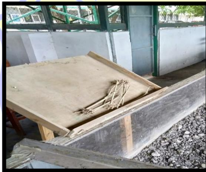
Gambar 3.7 Perlengkapan Penelitian, (a) Boks Bambu ukuran 40 cm x 30 cm, (b) Saringan ukuran 40 cm x 30 cm.
