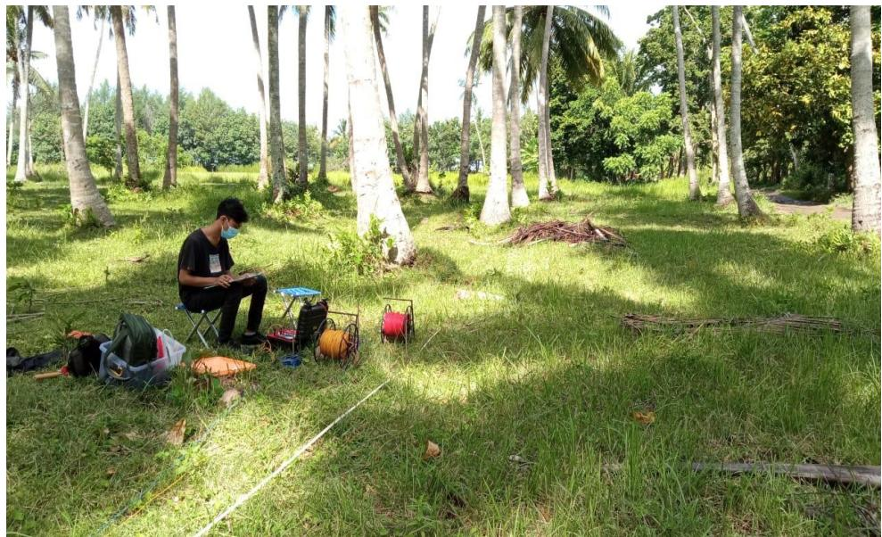
Mencatat data hasil penginjeksian alat *OJS Resistivity Meter V- RM 0219*
