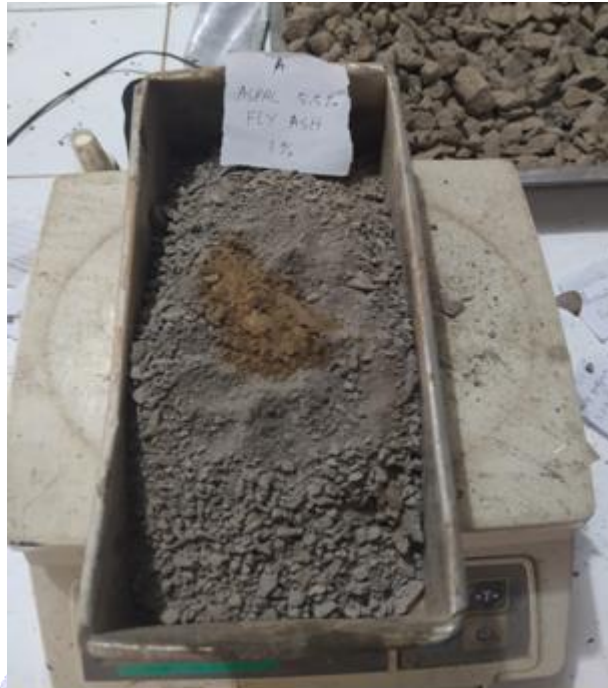
Penimbangan Campuran Agregat
