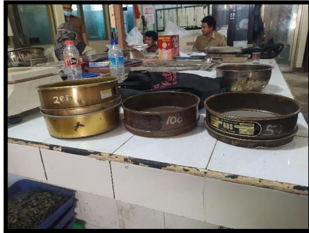
**Gambar 3.1** Saringan Standar ASTM
