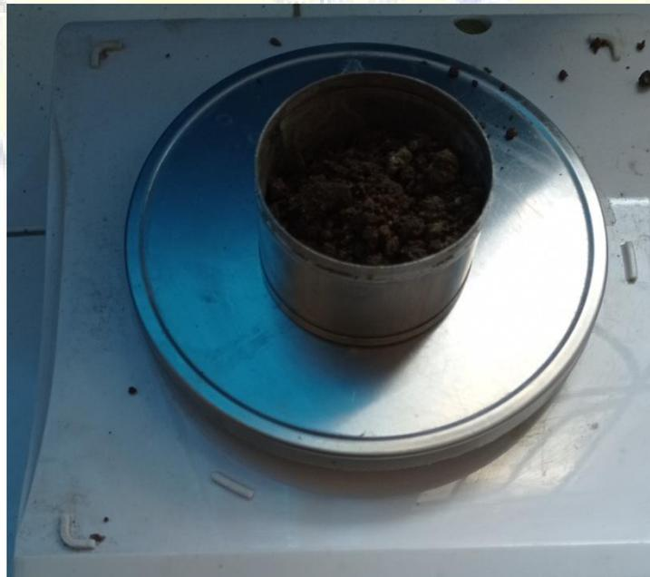
Penimbangan sampel tanah basah uji kadar air tanah asli
