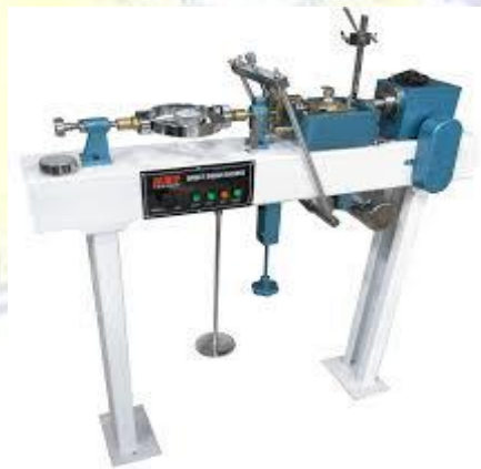
Gambar 3.8 Alat uji geser langsung (Direct Shear)
