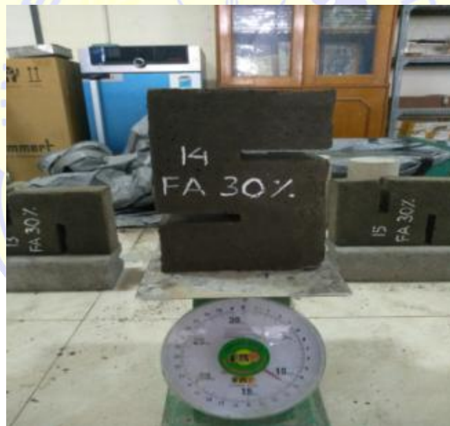
PENIMBANGAN BENDA UJI DOUBLE-L BETON KERING
