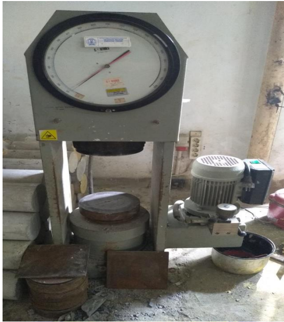
ALAT UJI KUAT TEKAN “COMPRESSION TESTING MACHINE (CTM)”
