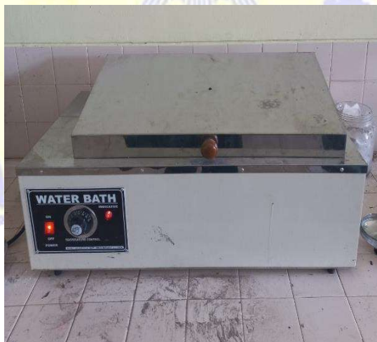
Gambar 3. 15 Satu set water bath
