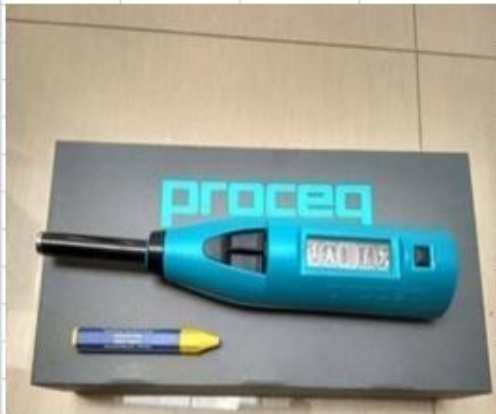
Alat Hammer Test
