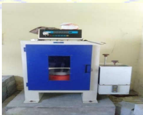
Gambar : 3.19. Compression Testing Machine Sumber : Dokumentasi Lab Mekanika Tanah, 2023
