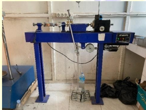
Gambar 3. 21 Alat uji kuat geser ( Direct shear electric )
