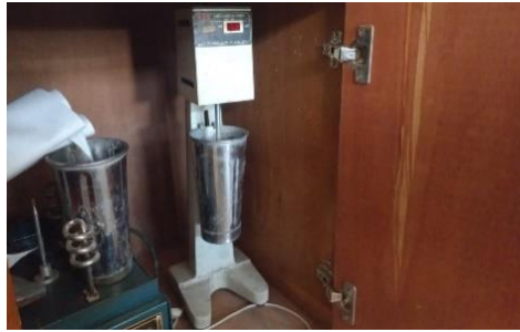
Gambar 3. 20 Pengaduk mekanik ( Mechanical stirrer )
