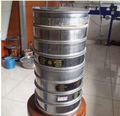
**Gambar 3.1** Saringan Standar ASTM
