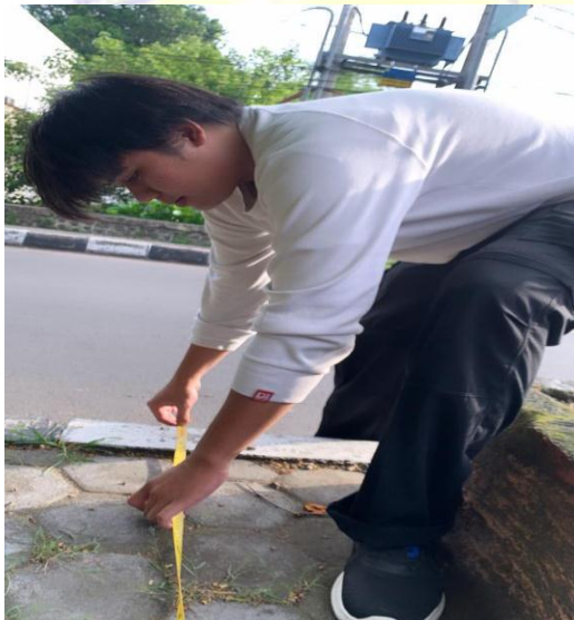
(Gambar D.3: Mengukur lebar median)
