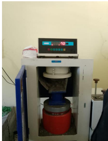
Benda uji 3 Fly Ash 35%
