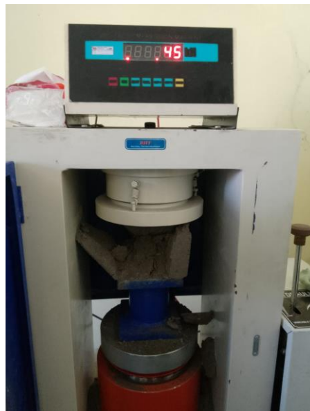
Benda uji 3 Fly Ash 50%
