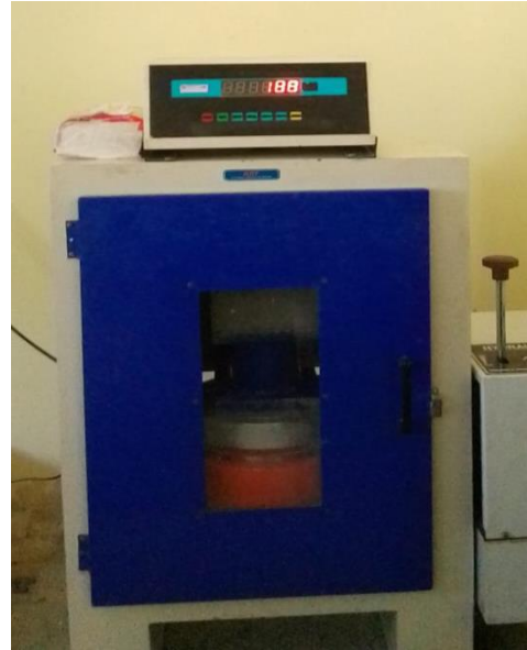
Benda uji 2 Fly Ash 15%
