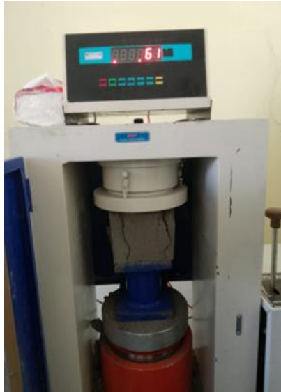
Benda uji 1 Fly Ash 35%
