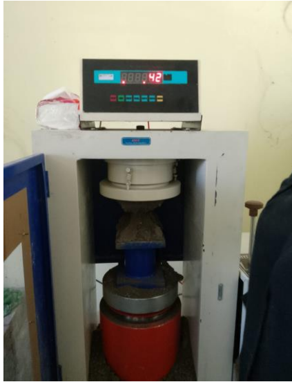
Benda uji 1 Fly Ash 50%
