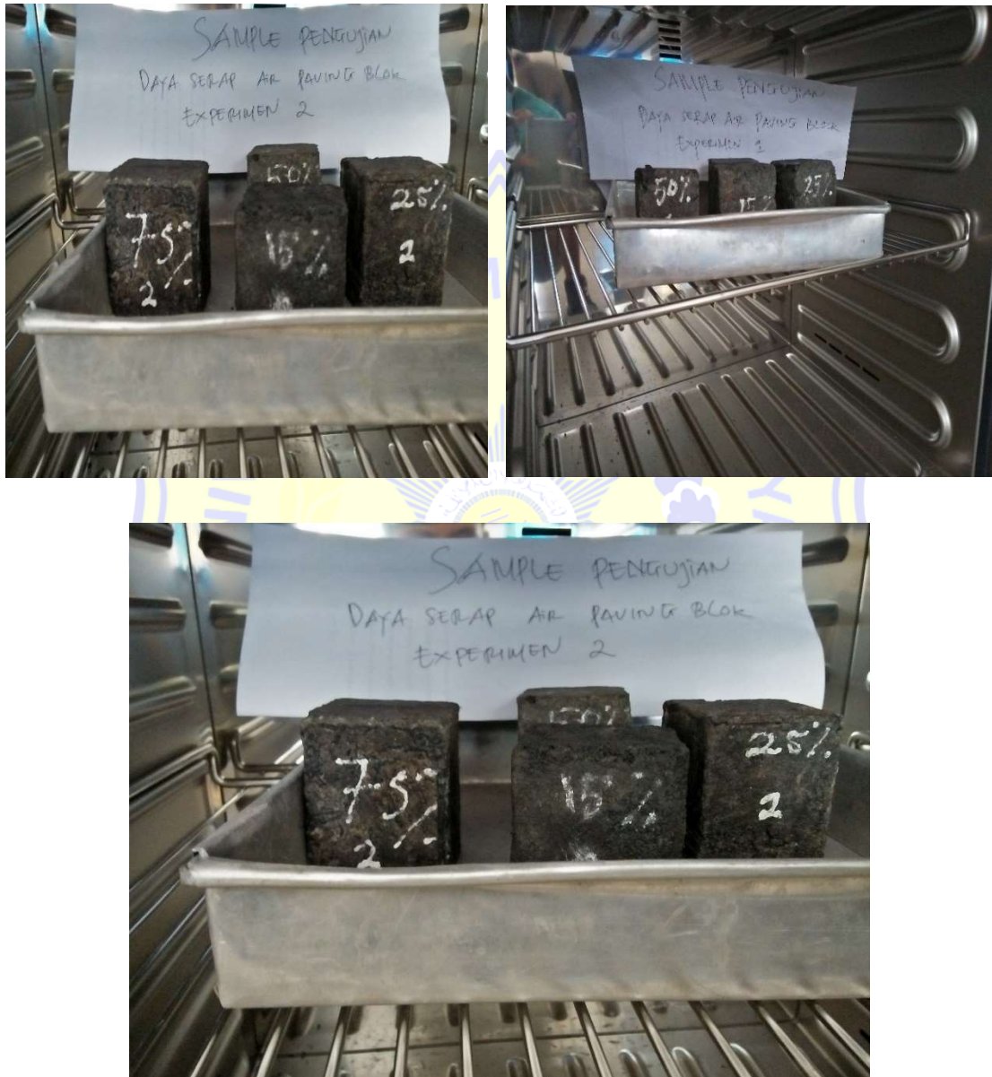
Gambar 26 : Proses pengujian daya serap air benda paving block
