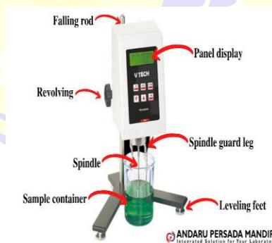
**Gambar 3.1** alat viscometer Brookfield tipe NDJ-8S
