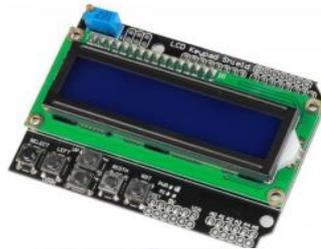
Gambar 2. LCD Karakter 1602 (Sumber: KelasRobot, 2015)
