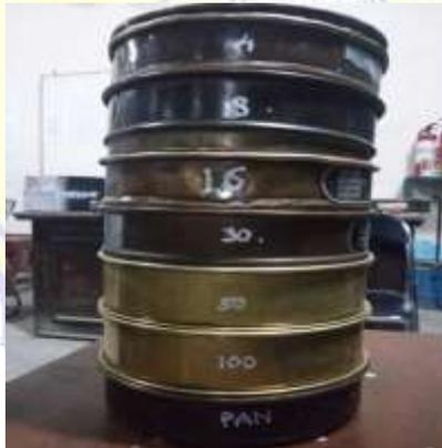
**Gambar 3.1** Saringan Standar ASTM
