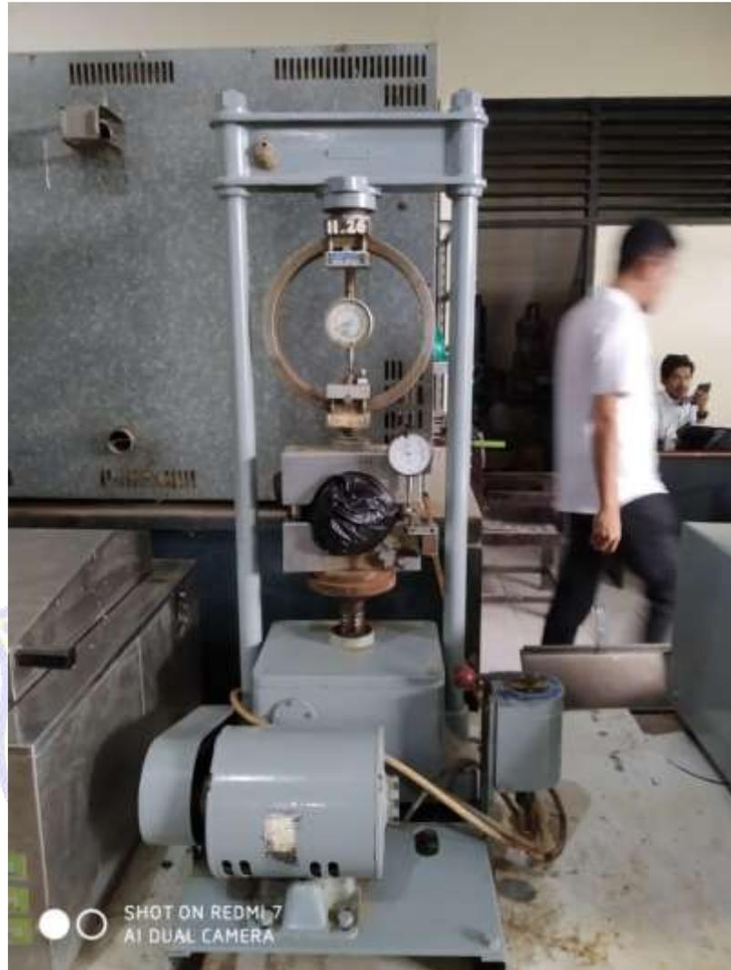
Gambar 3.4 *Marshall test*
