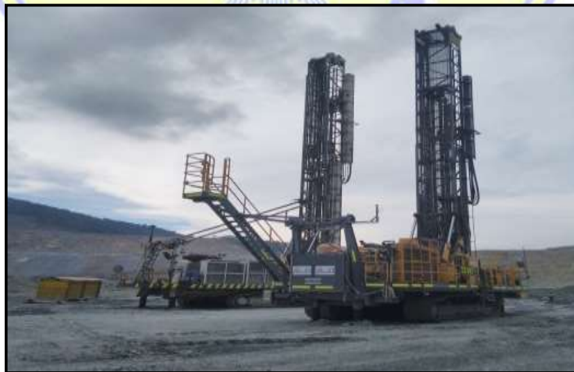
Gambar 7. Medium Drill Atlas-Copco PV235
