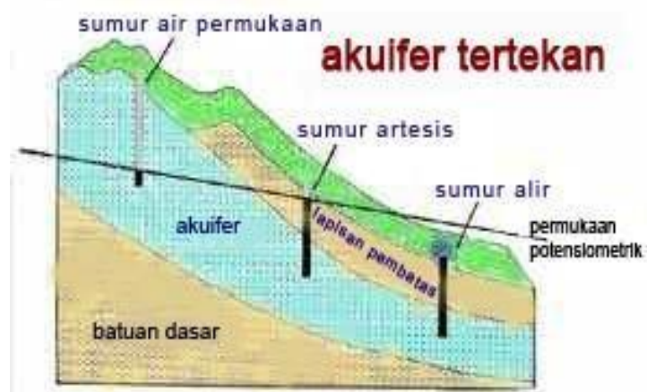
Gambar 2. 5 Akuifer tertekan ( Confined Aquifer ) (Wuryantoro, 2007)
