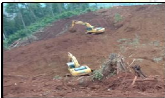
Gambar 2.3 Kegiatan Pengupasan Tanah penutup ( Top Soil Removal )
