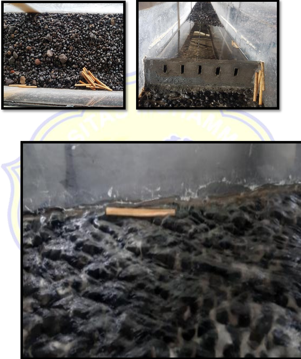
Gambar 3.24 Kondisi debris kayu di Sabo Dam, (a) Hulu, (b) sabo dam, (c) hilir
