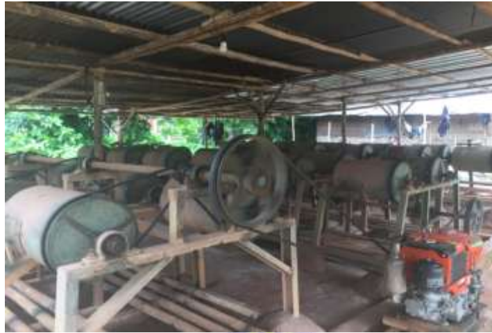
Gambar 5: Mesin Pengolah Matrial Tambang (gelondong)
