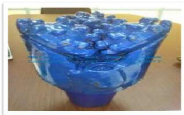
**Gambar 2.13** *Three Cone Bit*
