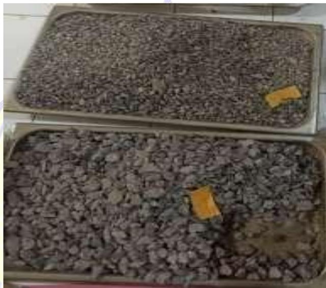
**Gambar 3.15** Agregat 3/4" dan Agregat 3/8"
