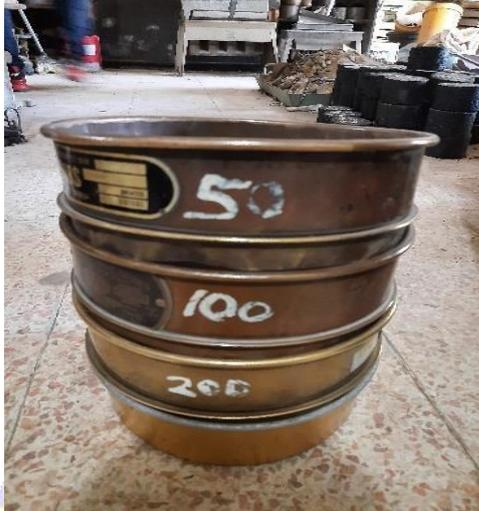
**Gambar 3.1** Alat uji saringan standar ASTM
